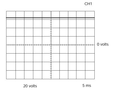
This is the typical CV output voltage generated from a properly operating machine. Note that each vertical division represents 20 volts and that each horizontal division represents 5 milliseconds in time.
